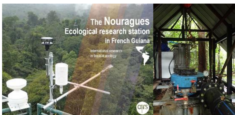
Figure 23 - Example of a 10 kW hydro turbine at CNRS ANAEE Nouragues station.
