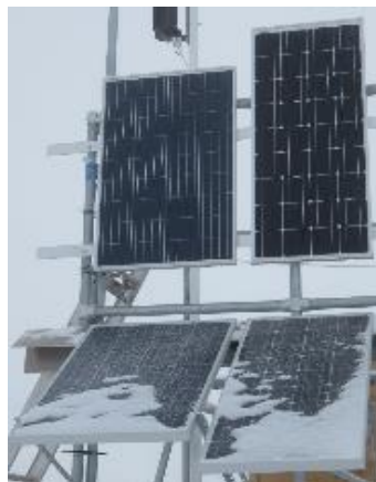
Figure 72 - Snow deposition on 36° tilted solar panels
