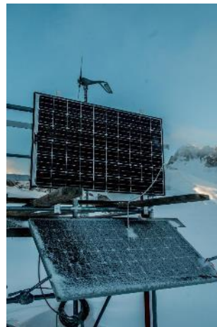
Figure 56 - Two monofacial 250Wp evaluated solar panels (here during installation). Source: ISTerre.
