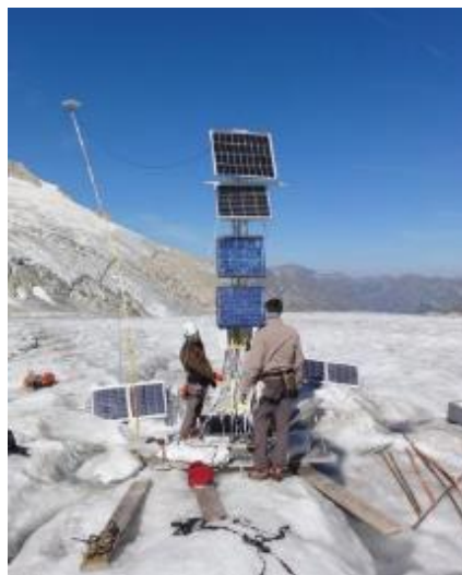
Figure 5 – Example of isolated scientific station powered with photovoltaic solar panels. Source: RESIF-GNSS network. ISTerre laboratory.
