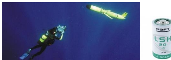
Figure 37 - An example of use Lithium Sulfuryl Chloride (primary non rechargeable) cell in oceanic domain, RI's feedbacks in survey.
