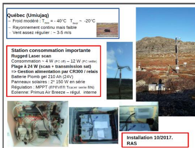
Figure 87 - Additional example of the HAWT use on field (Quebec). Source: IGE
